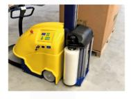
Film tension adjustment: mechanical brake.
