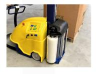
Film tension adjustment: mechanical brake.
